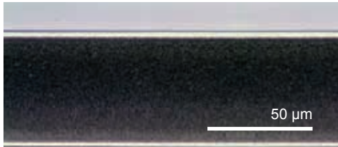
Tempered glass 0.55 mm thickness, 42 µm DOL. Side view
